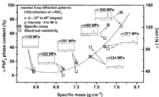
Figure 3  $\alpha$ - $\text{PbF}_2$  phase content and electrical resistivity at 298 K as a function of specific mass of  $\beta$ - $\text{PbF}_2$  pellets pressed at different loads: 148 MPa, 222 MPa, 297 MPa, 334 MPa, 371 MPa, 408 MPa, 480 MPa and  $\sim$ 500 MPa. XRD patterns of the (103) reflection  $\alpha$ - $\text{PbF}_2$  are shown as a function of the load.
