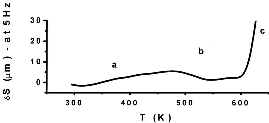
Figure 5 Bottom: Room temperature to 673 K Dynamic-Mechanical Analysis of  $\beta$ -PbF<sub>2</sub> pressed at 297 MPa; Top: SEM micrographs of fractured surfaces and room temperature XRD patterns of the as pressed pellet (a); after heating at 573 K (b); after heating to 633 K, cooling to room temperature and further heating to 573 K.
