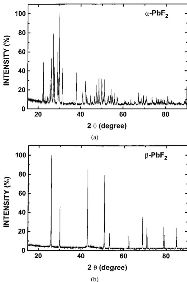
Figure 1 XRD patterns of  $\alpha$ - $\text{PbF}_2$  (a) and  $\beta$ - $\text{PbF}_2$  (b).
