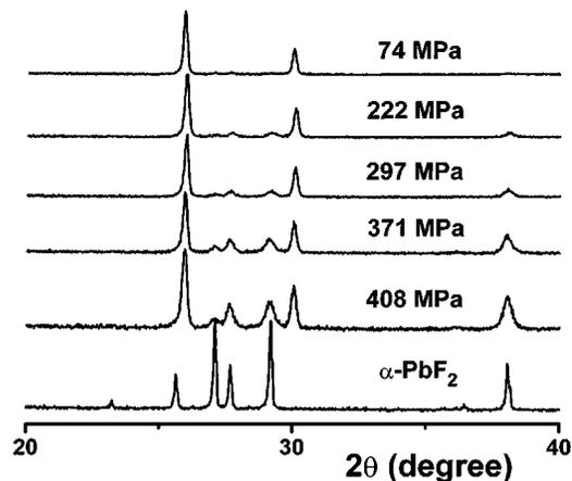
Figure 2 XRD patterns of  $\beta$ - $\text{PbF}_2$  pellets pressed at different loads: 74 MPa, 222 MPa, 297 MPa, 371 MPa, 408 MPa; pattern at the bottom:  $\alpha$ - $\text{PbF}_2$  as prepared.
