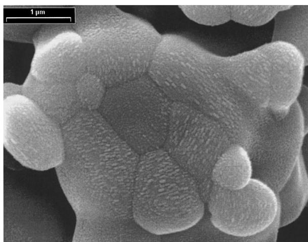
Figure 8 SEM micrograph of a fractured surface of  $\text{PbF}_2$  pellet pressed at 74 MPa and heated to 533 K showing grains with oriented crystals.
