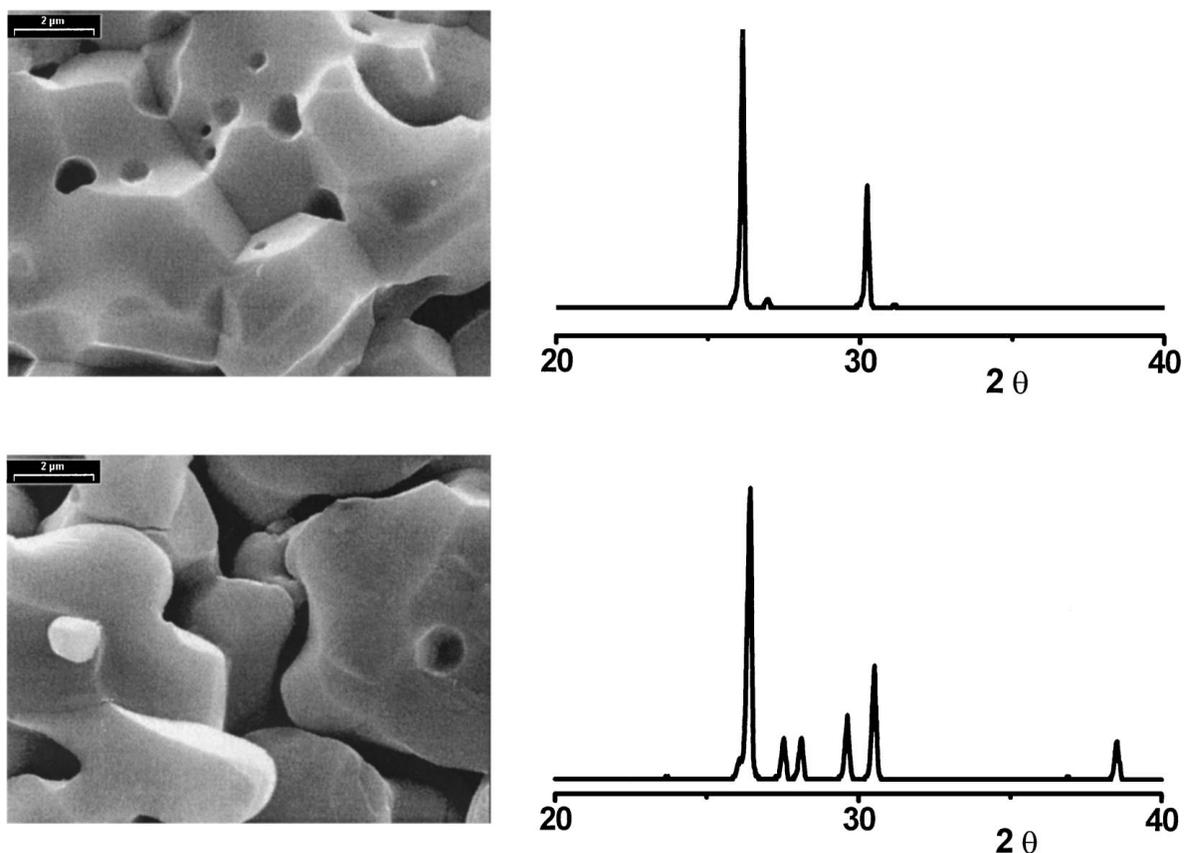
Figure 6 SEM micrographs of fractured surfaces and room temperature XRD patterns of the PbF<sub>2</sub> pellet: after heating to 673 K, cooling to room temperature and heating to 573 K (a); after pressing at 74 MPa and heating to 573 K (b).
