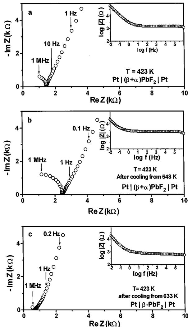
Figure 9 Impedance spectroscopy diagrams (Nyquist and Bode) of  $\text{PbF}_2$  pellets measured at 423 K: after pressing (a); after heating to a temperature below the  $\alpha \rightarrow \beta$  phase transition (548 K) and cooling to 423 K (b); and after heating to a temperature above the  $\alpha \rightarrow \beta$  phase transition (633 K) and cooling to 423 K.
