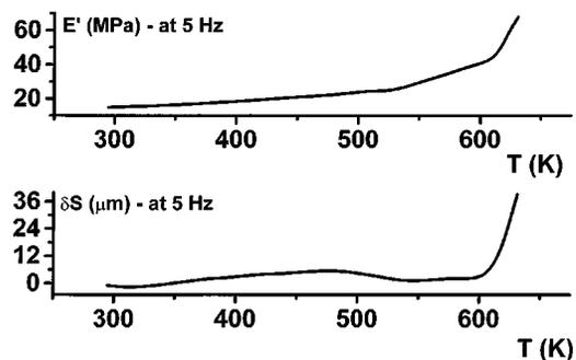
Figure 4 Room temperature to 633 K Dynamic-Mechanical Analysis of  $\beta$ - $\text{PbF}_2$  pressed at 297 MPa.
